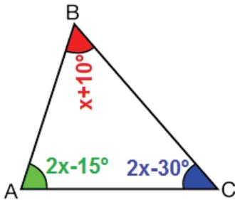
$$\begin{aligned} \hat{A} + \hat{B} + \hat{C} &= 180^\circ \\ 2x - 15^\circ + x + 10^\circ + 2x - 30^\circ &= 180^\circ \\ 2x + x + 2x &= 180^\circ + 15^\circ - 10^\circ + 30^\circ \\ 5x &= 225^\circ \\ x &= \frac{225^\circ}{5} = 45^\circ \\ x &= 45^\circ \quad \text{Solución} \end{aligned}$$
